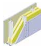
Cloison séparative SAD 160 Placo® DuoTech® 25 R_w (C; C_{tr}) = 69 (-3; -10) \text{ dB}
